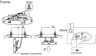
5. Disassembly process: one hand to hold the speaker assembly and push it up slightly, then use a hook to hook the edge of grill and rotate counterclockwise till the speaker assembly apart from the frame.
